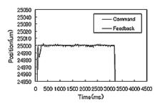
Fig. 1 Typical positioning precision when loaded at 86kN
